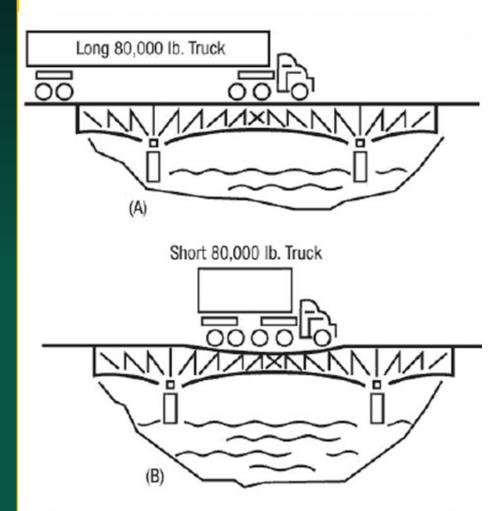
Axle spacing is as important as axle weight in designing bridges. In Figure A, the stress on bridge members as a longer truck rolls across is much less than that caused by a short vehicle as shown in Figure B, even though both trucks have the same total weight and individual axle weights. The weight of the longer vehicle is spread out, while the shorter vehicle is concentrated on a smaller area.
