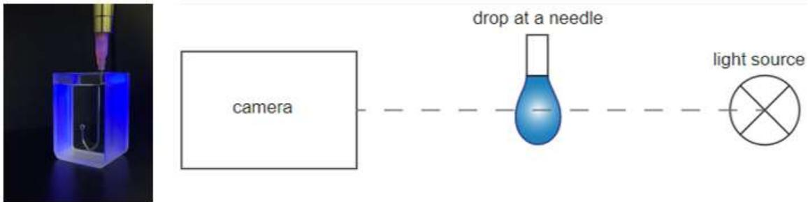
optical contact angle measuring and contour analysis called the “Pendant Drop Method”.
